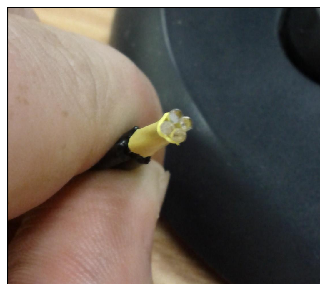
b) A prototype fiber diamond utilizing large core PMMA multimode fibers.
