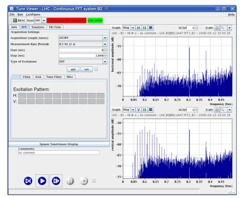
Coupling measurement benefited from the chirp excitation using the exciter of the RF transverse damper (see next slide)
