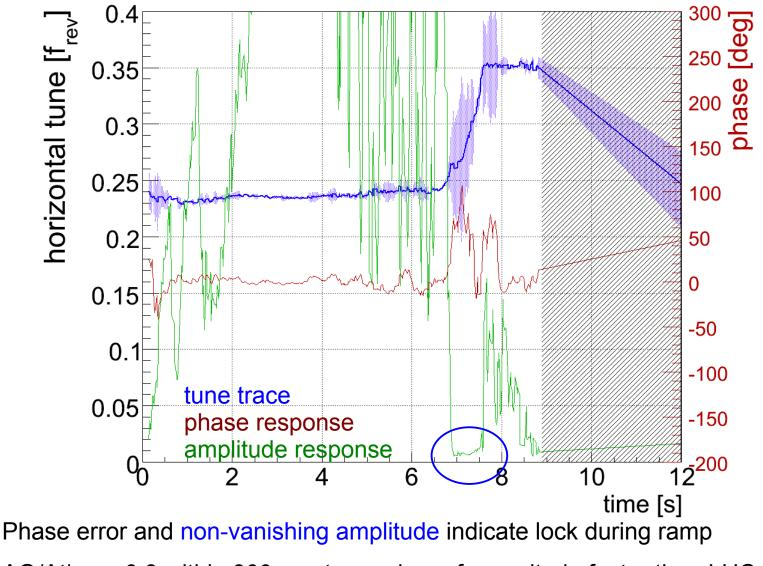
$\Delta Q/\Delta t|_{max} \approx 0.3$  within 300 ms, two orders of magnitude faster than LHC req.  $f_{rev} \approx 43$  kHz
