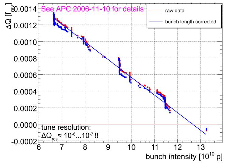
Using Sacherer's impedance approximation:  $Z_{eff} \approx 21.54 \text{ M}\Omega/\text{m}$
