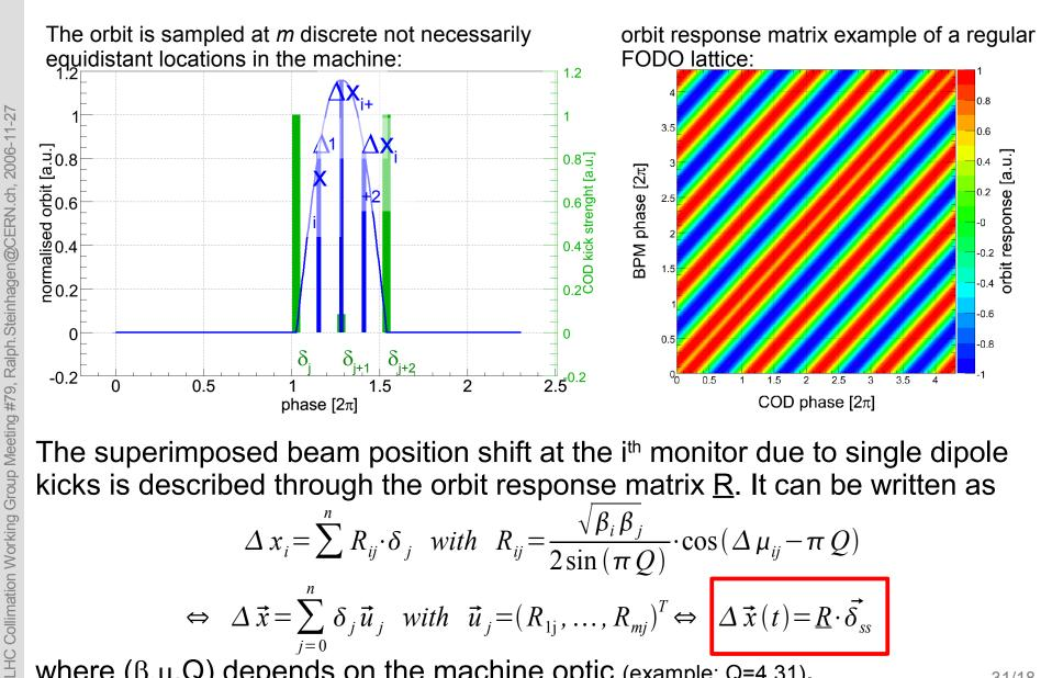
The superimposed beam position shift at the i<sup>th</sup> monitor due to single dipole kicks is described through the orbit response matrix R. It can be written as
