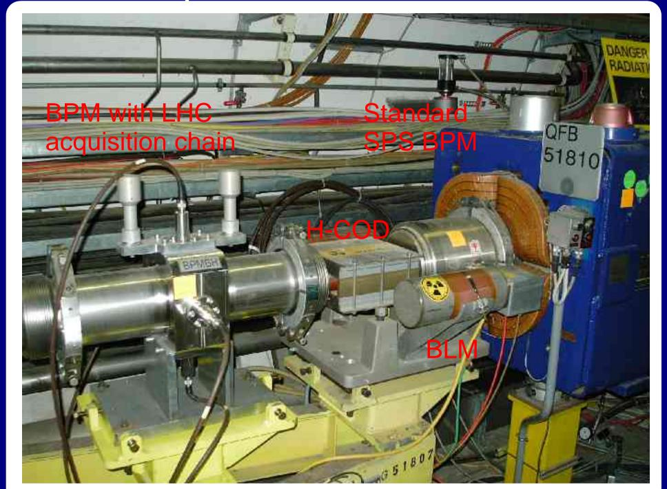
For the feedback tests, six BPMs with full LHC BPM acquisition system but ~ 40% larger (SPS) aperture were available.
